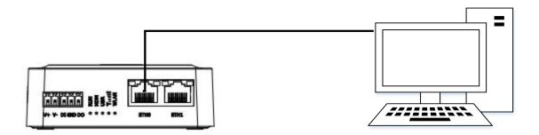
Connect an standard Ethernet cable to the port marked ETH0~ETH1 at the front of the R1510 Router, and connect the other end of the cable to your computer.
