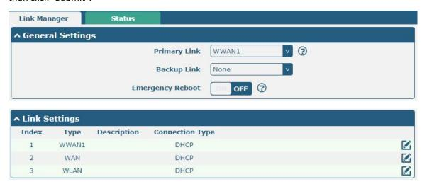
Click the right most of edit button of WWAN1 to set its parameters according to the current ISP.
