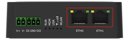
There are two Ethernet ports on R1510, including ETH0 (WAN/LAN), and ETH1. Each has two LED indicators. The yellow one is a link indicator but the green one doesn't mean anything. For details about status, see the table below.
