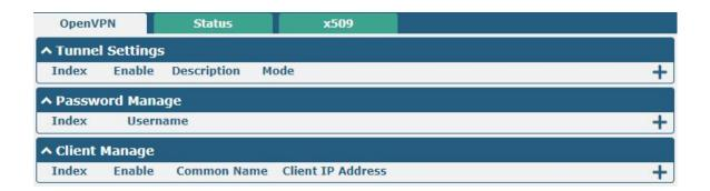
Click to add OpenVPN tunnel settings. The maximum count is 5. By default, the mode is "P2P". The window is displayed as below when choosing "P2P" as the mode.
