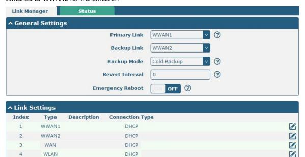
Click the right most of edit button of WWAN1 to set its parameters according to the current ISP.
