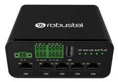
• 1 x 2-pin 3.5 mm male terminal block with lock for power supply
