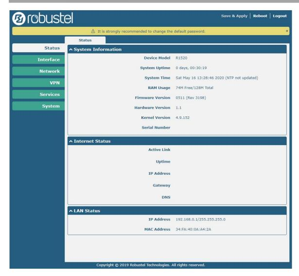
In the home page, the user can save the configuration, restart the router, log out, and so on.
