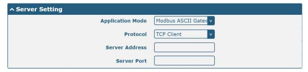
When selecting "ModBus ASCII Gateway" as the application mode and "TCP Server" as the protocol, the window is as follows:
