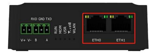
There are two Ethernet ports on R1511, including ETH0 (WAN/LAN), and ETH1. Each has two LED indicators. The green one is a link indicator but the yellow one doesn't mean anything (always off). For details about status, see the table below.
